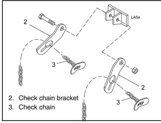
Figure 9. Check Chain Adjustment
